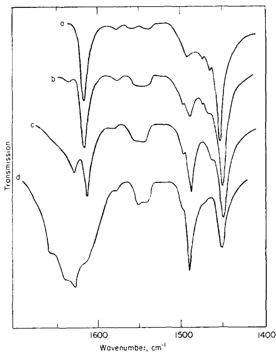
FIG. 5. Infrared spectra of pyridine adsorbed on Zn-X. Zn-X was pretreated at 450°C in vacuum. a, After evacuation of pyridine at 200°C; b, a + H 2 O at 0.1 mm and evacuated at 200°C for 30 min; c, b + additional amount of water; d, c + additional amount of water (pressure of water was 0.1 mm at 200°C).
